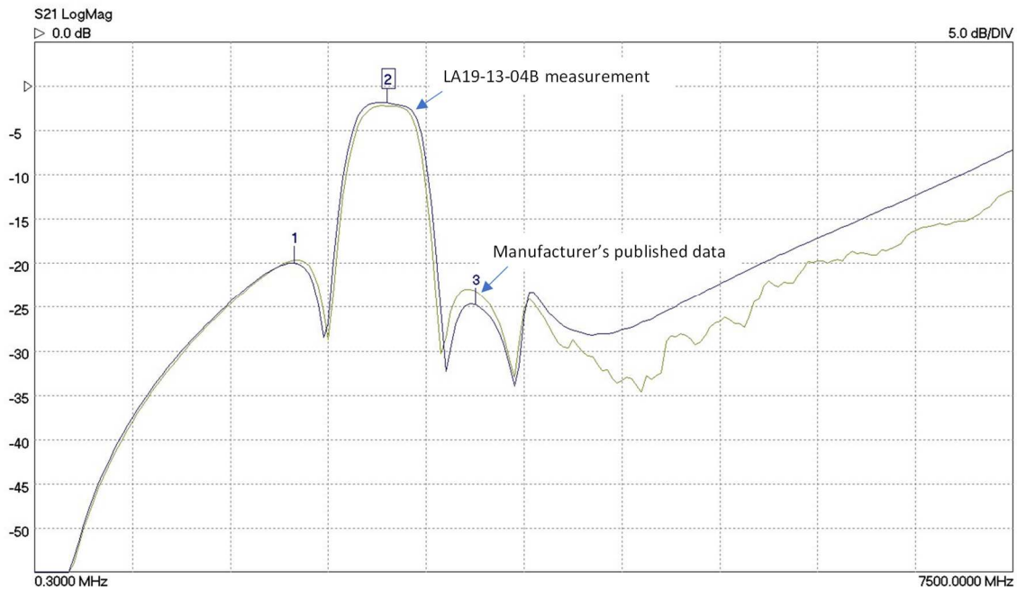
Figure 7a: Bandpass filter (BFCN-2700+) S21 measurement
