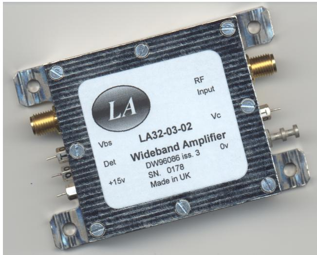
The LA32-03-02 is a power amplifier intended for use in applications requiring large bandwidths. It is well suited for driving optical modulators as its output stage can cope well with low impedance loads. It incorporates output level control, monitor, and bias-T.
