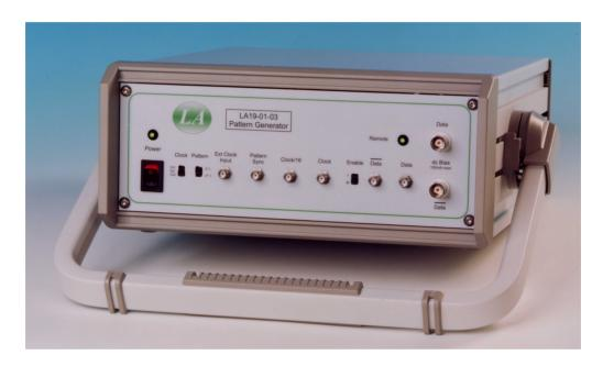
The LA19-01-03 is a pseudo random pulse pattern generator capable of operation up to 3 Gb/s. It provides a fast rise time and low pulse distortion. The unit can accommodate two internal clock generators and supports an external clock input. It provides a clean pulse output suitable for applications such as optical communications, fast pulse amplifiers and high speed logic circuits development. Remote control is via an IEEE488 interface.
