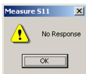
If the data link is interrupted reset the VNA (red button on rear panel) and re-start the UI software ('Tools' menu)
