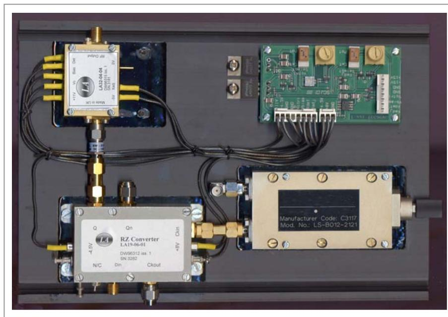
The LA19-08-01 is an RZ evaluation kit incorporating LA Techniques' NRZ to RZ converter and RZ driver amplifier together with a mechanical phase adjuster in one ready to use unit. It is intended for evaluation purposes and includes a power supply regulator with manual or electronic (select via an on-board switch) adjustment of the output level and output pulse width. The key features are as follows:
