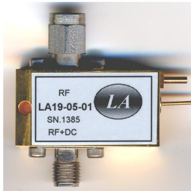
The LA19-05-01 is a broad band dc bias insertion tee. It is intended to pass high speed digital signals with little distortion. It provides a well controlled response extending from 50 kHz to over 40 GHz. It provides a pulse rise time of less than 10 ps and is able to support a maximum dc current of up to 200 mA. The LA19-05-01 is ideally suited for 40 Gb/s systems and other broad band applications
